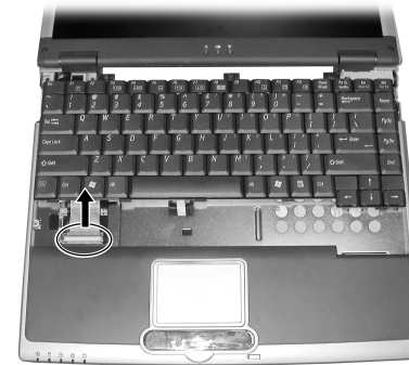
Figure 2-5 Disconnect the cable
