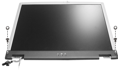
Figure 2-28 Remove LCD cover
