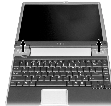
Figure 2-3 Remove the speaker cover
