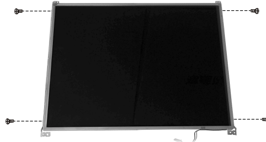
Figure 2-33 Free the LCD panel
