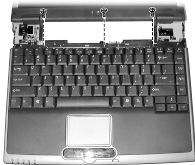
Figure 2-4 Remove three screws
