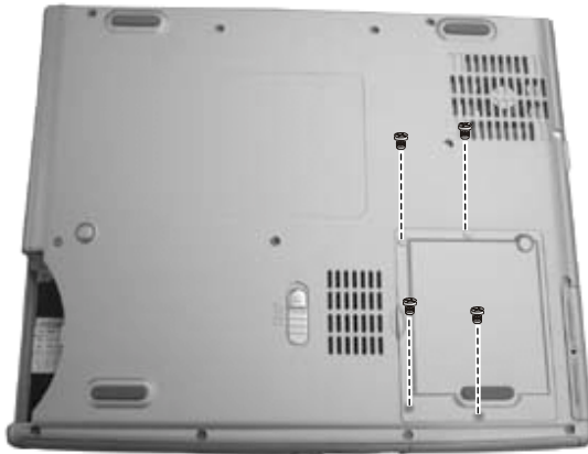
Figure 2-13 Remove the SO-DIMM Cover
