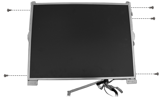
Figure 2-24 Remove the five screws
