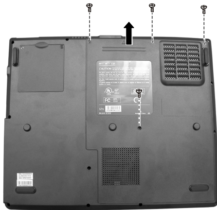
Figure 2-1 Remove the four screws
