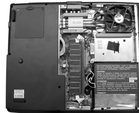
Figure 2-2 Remove the battery pack
