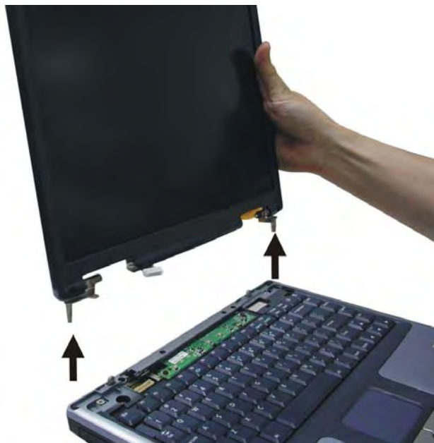
Figure 5-8: Lifting off the display assembly
