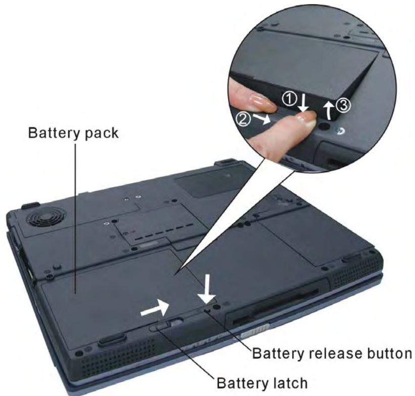
Figure 5-1: Removing the battery
