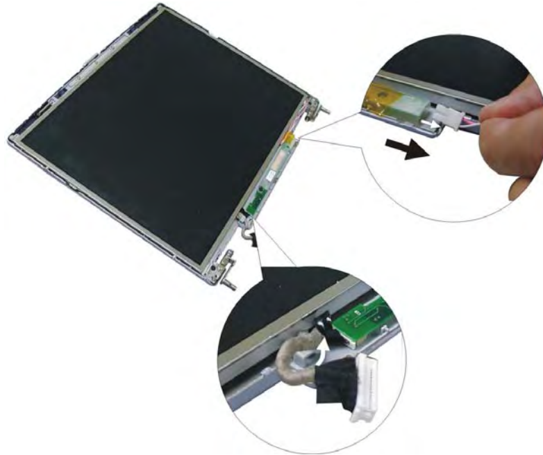
Figure 5-12: Detaching the FL inverter board
