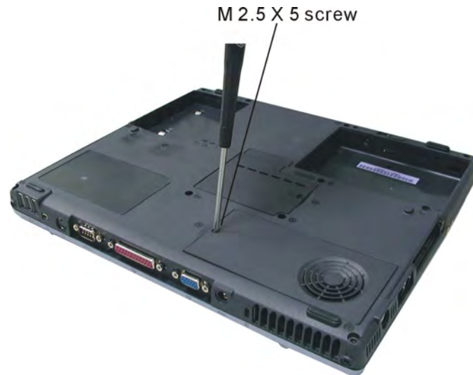
Figure 5-32: Removing the CPU compartment cover
