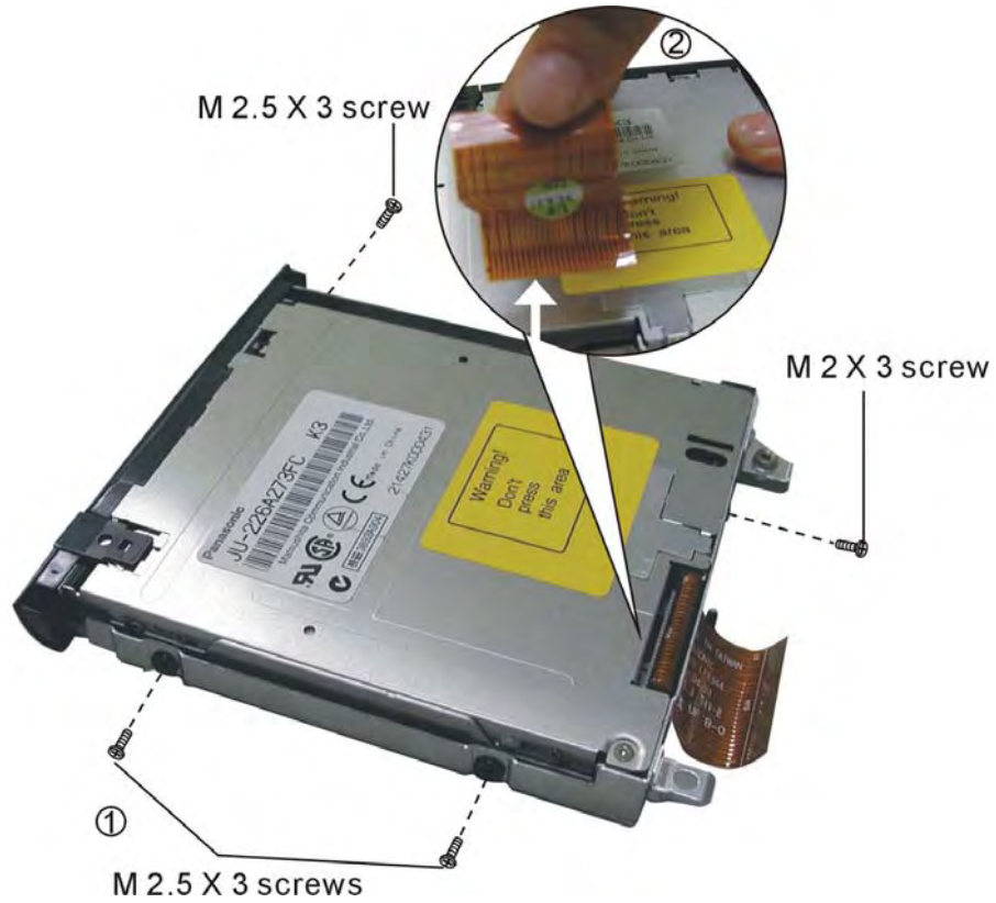
Figure5-29: Removing the FDD brace and cable
