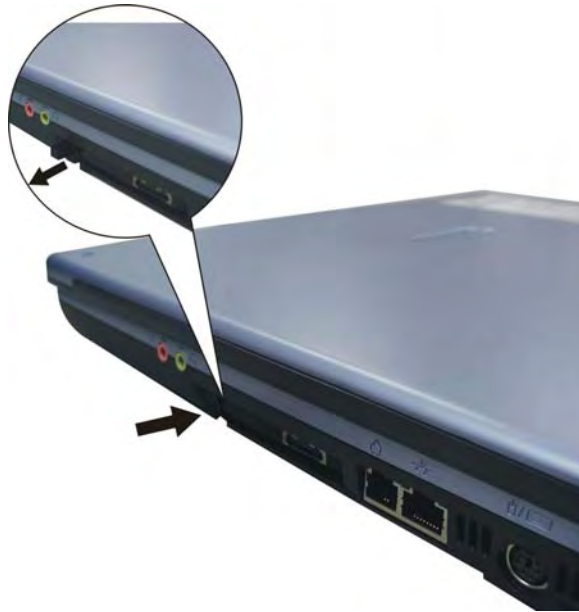
Figure 5-2: Ejecting a PC card (1/2)
