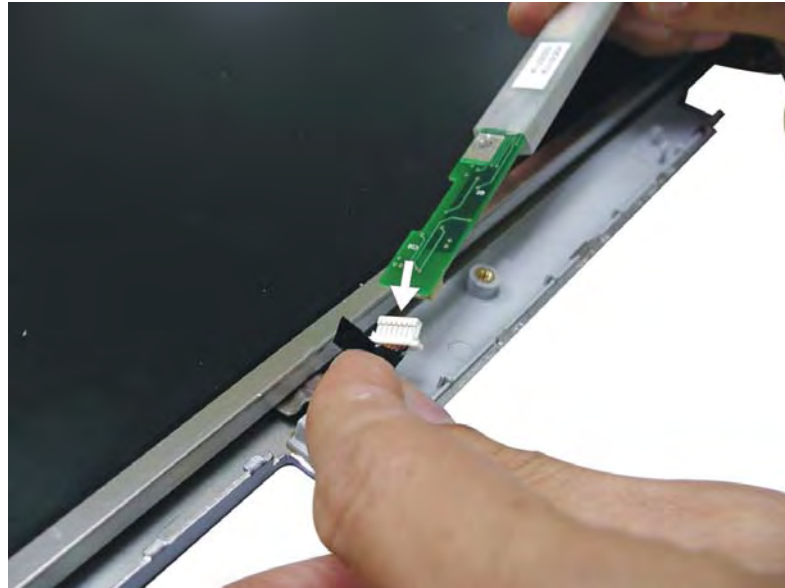
Figure 5-13: Detaching the FL FPC
