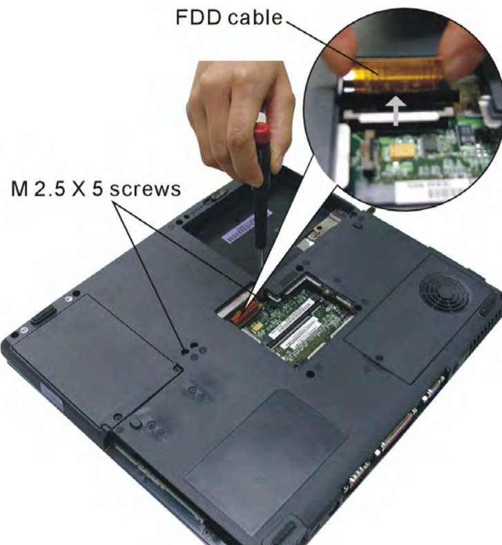
Figure 5-28: Detaching the FDD
