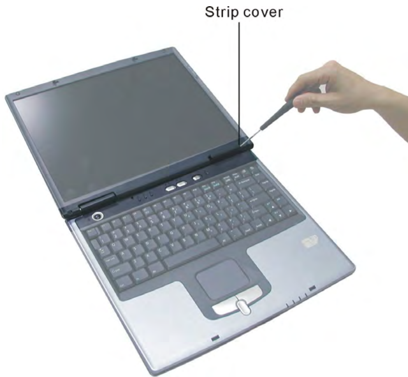
Figure 5-5: Removing the strip cover
