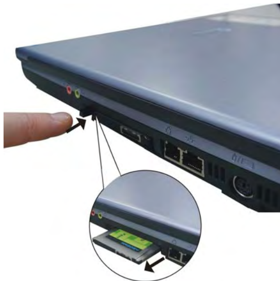
Figure 5-3: Ejecting a PC card (2/2)
