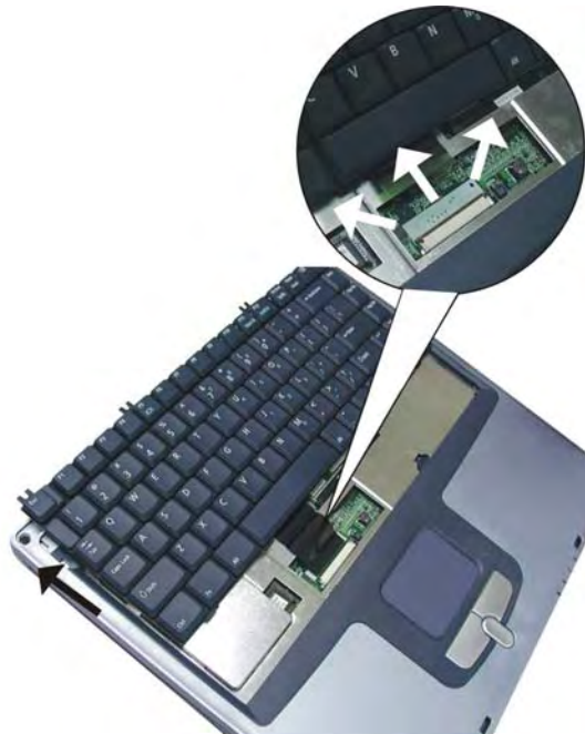
Figure 5-17: Removing the keyboard
