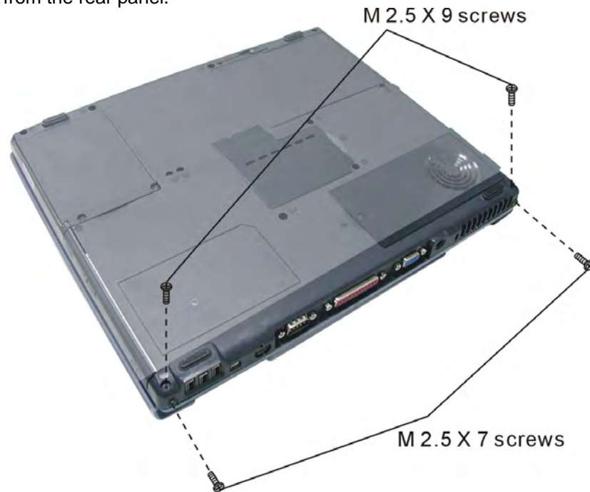
Figure 5-7: Removing two screws securing the display assembly
