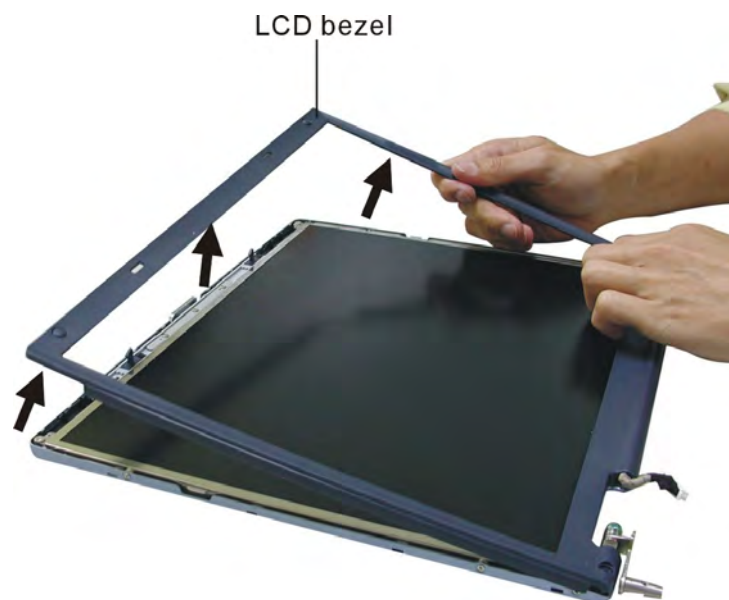
Figure 5-10: Removing the LCD bezel
