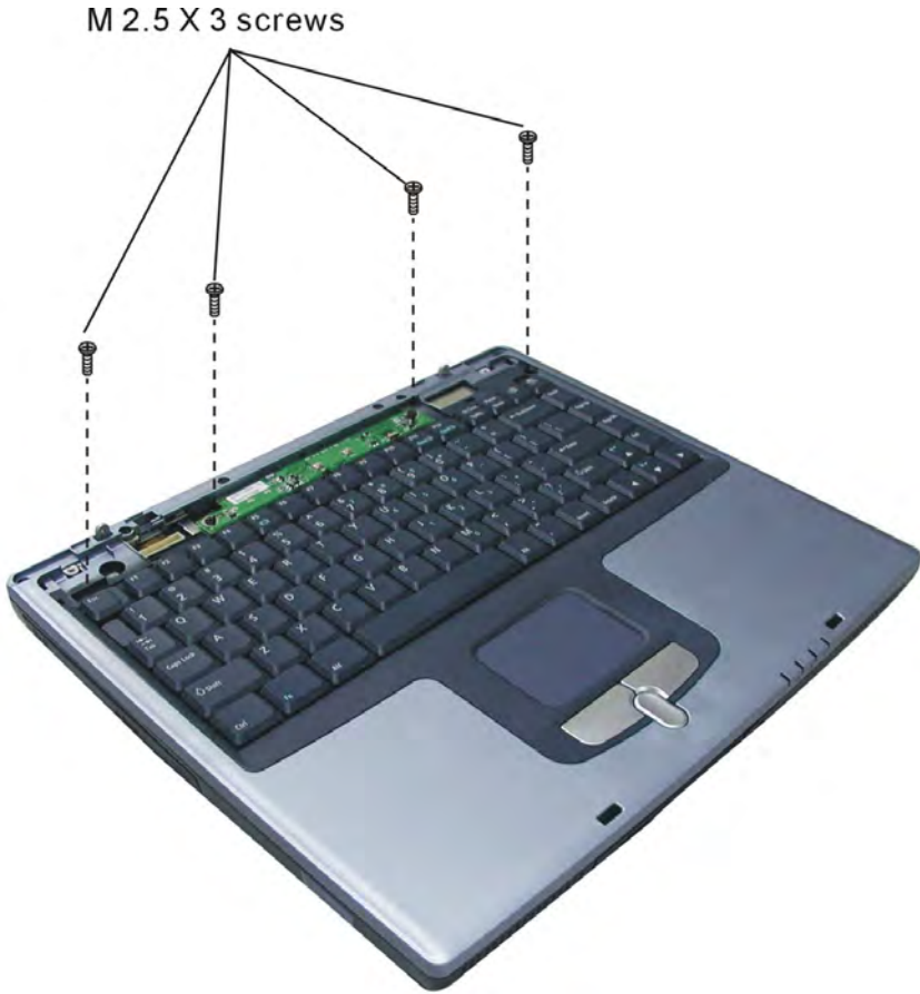
Figure 5-16: Removing four screws securing the keyboard
