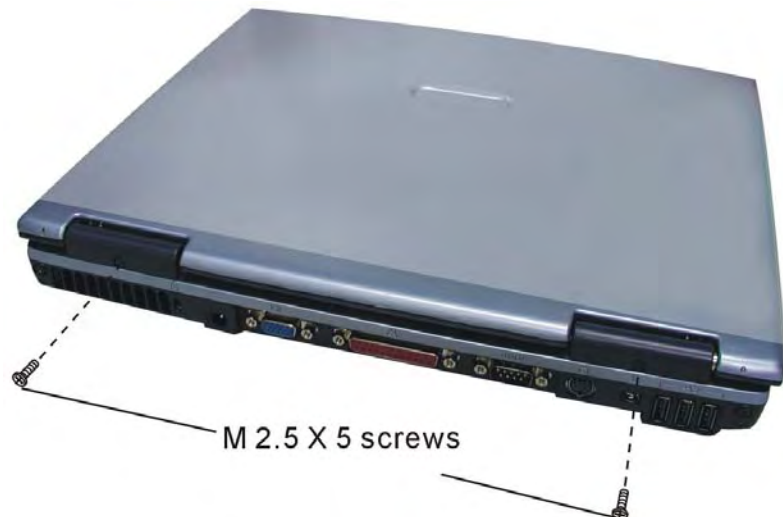
Figure 5-4: Removing two screws securing the strip cover
