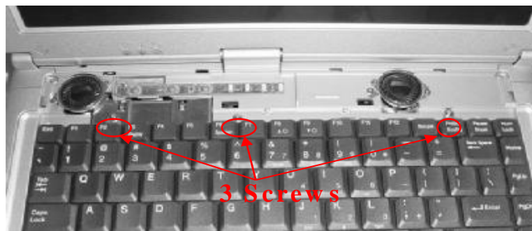
Figure 5-4 Remove Three Screws on the Keyboard
