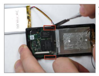
• Disconnect the faceplate from the device by depressing the two tabs located near the middle of each of the sides using a metal spudger.
