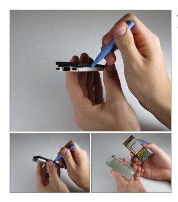
• Work your way around the Zune until the back cover comes free. Remove the back plate and set it aside.
