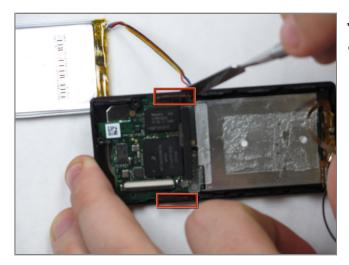
• Disconnect the faceplate from the device by depressing the two tabs located near the middle of each of the sides using a metal spudger.
