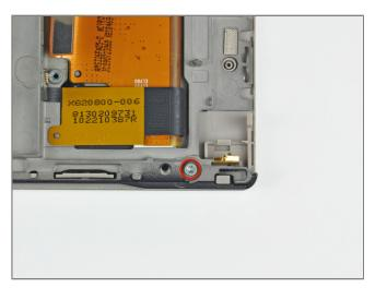
• Remove the single T5 Torx screw securing the front case to the inner chassis.
