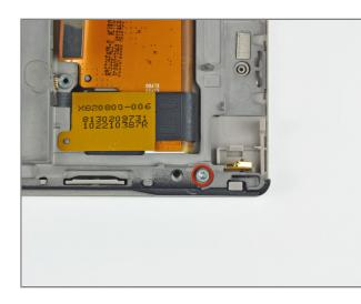
• Remove the single T5 Torx screw securing the front case to the inner chassis.
