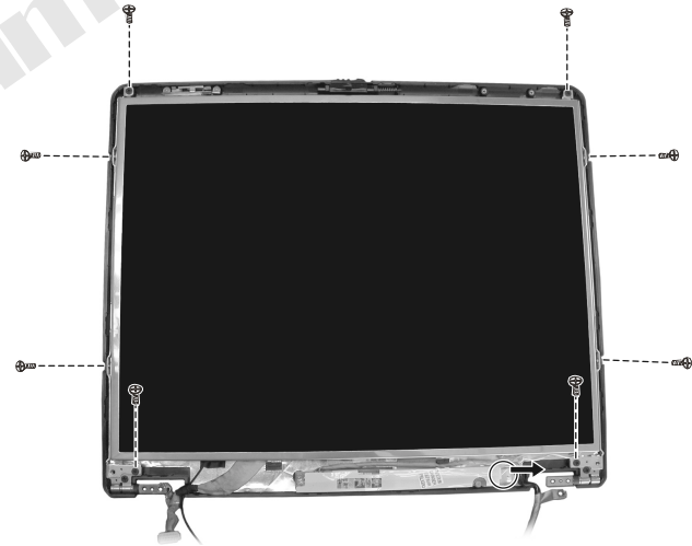
Figure 2-19 Remove the eight screws and disconnect the cable
