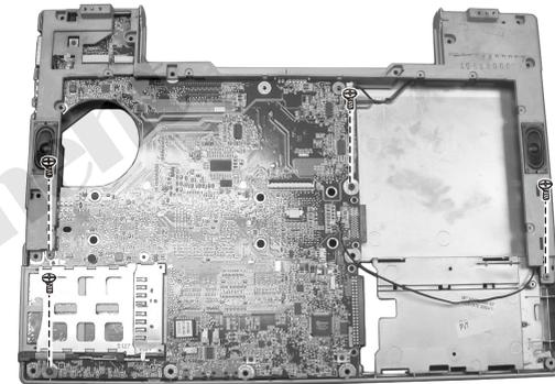
Figure 2-28 Remove the four screws
