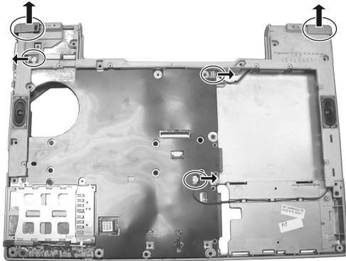
Figure 2-27 Disconnect the cables and separate the rear covers
