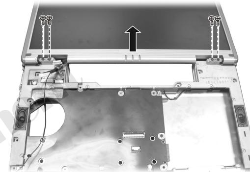
Figure 2-19 Free the LCD assembly
