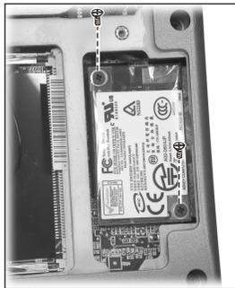
Figure 2-12 Remove two screws
