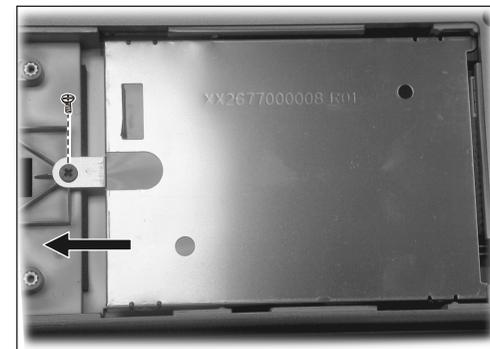
Figure 2-8 Remove HDD module
