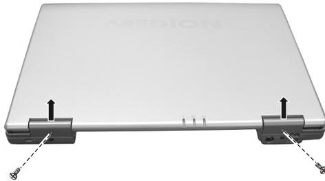
Figure 2-18 Free the two hinge covers
