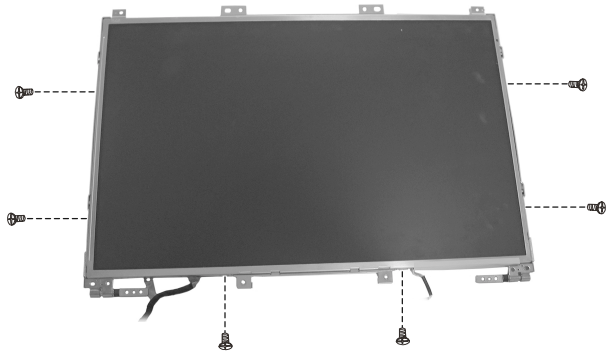
Figure 2-27 Remove the six screws
