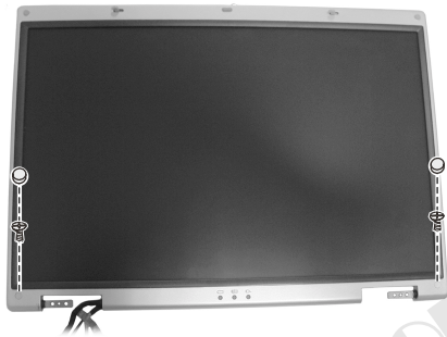
Figure 2-25 Remove LCD cover
