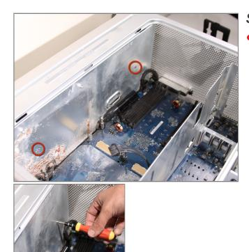
• Remove the 2 Philips screws holding the power supply cover on.
