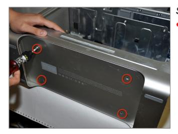
• Remove the 4 Philips screws on the underside of the computer case.
