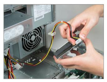
• Remove the multicolored cable by grasping the plastic connector on either side and pulling with substantial force.
