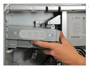
• Remove the optical drive by pulling the drive away from the front of the computer and out.
