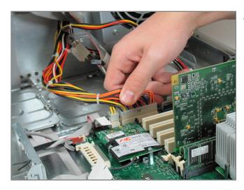
• Disconnect the power supply cables from the mother board by pressing in the tab on the back of the connector as shown.
