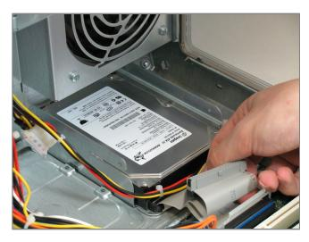
• Remove the flat ribbon cable by pulling with substantial force.
