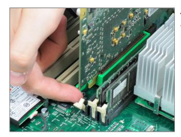
• Before lifting the card out, this small plastic tab needs to be pulled back there by releasing it entirely.
