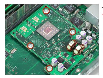
• Remove the four screws holding the CPU to the motherboard.
