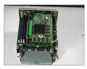
Remove the screw attaching the video card to the logic board.
