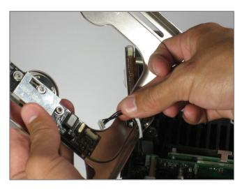
• Slowly lift the plate off the cube and disconnect the power cord.
