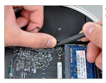
• To disconnect the optical drive thermal sensor, pinch its cables between your thumb and a spudger and pry the spudger upward to lift the connector up and out of its socket on the logic board.
