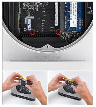
• To remove the logic board, two cylindrical rods must be inserted into the holes highlighted in red. Inserting instruments into any logic board holes other than the ones highlighted in red may destroy the logic board.
