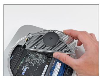
• Remove the antenna plate from the mini.
