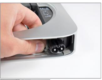
• Pull the AC-In socket retainer away from the side of the outer case and remove it from the mini.
