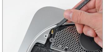
• Use the tip of a spudger to carefully pry the antenna connector up off the AirPort/Bluetooth board.
