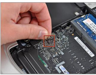
Carefully pull the wires for both hard drive thermal sensors upward to lift their connectors up and out of the sockets on the logic board.
