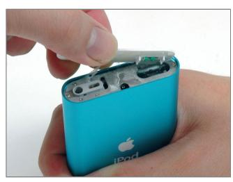
• Lift the top bezel off of the iPod.
