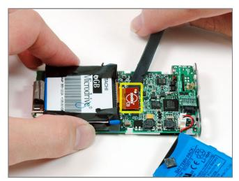
Use a spudger or the tip of your finger to carefully disconect the orange hard drive ribbon from the logic board.
