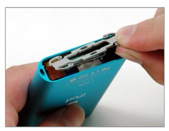
• Lift the metal retaining bracket out of the iPod.
