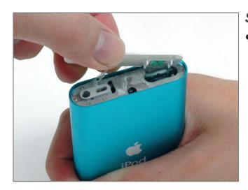
Step 3Lift the top bezel off of the iPod.
