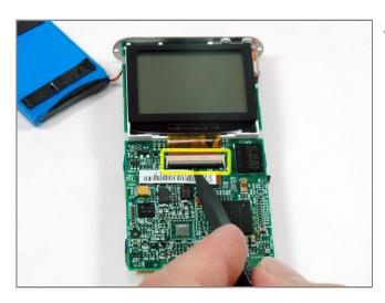
• Use a spudger to flip up the black plastic tab holding the orange display ribbon in place. The black tab will rotate up 90 degrees, releasing the ribbon cable.
