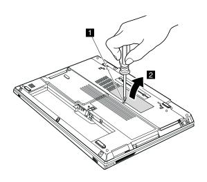
Note: Loosen the screw 1 but do not remove it.
