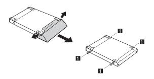
When installing: Make sure that the HDD connector is firmly connected.
