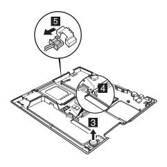
When installing: Make sure that you fasten the connector firmly.
