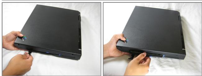
To reassemble, place the floppy disk drive back into its bay the way it was facing before
