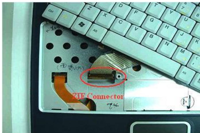
Figure 2-3 Remove keyboard
