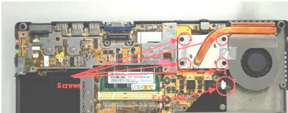
Figure 2-5 Remove heat sink plate and Fan
