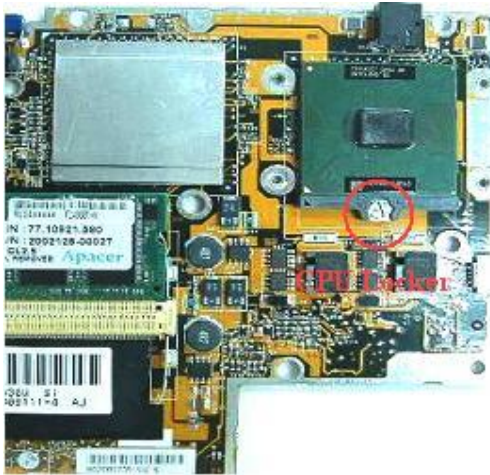
Figure 2-6 Remove CPU
