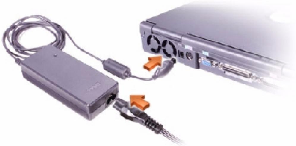
The AC adapter converts AC power to the DC power required by the computer. You can connect the AC adapter with your computer turned either on or off.
