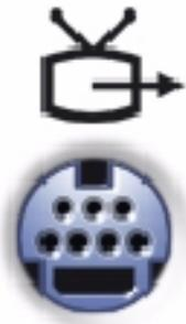
Connects your computer to a TV. Also connects S/PDIF capable devices using the TV/digital audio adapter cable.
