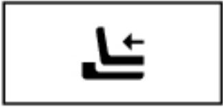
Connects the optional docking device. A docking device allows you to easily use external devices with your computer, such as an external keyboard, mouse, and monitor.
