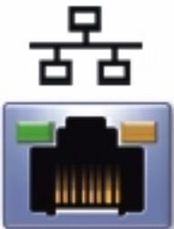
Connects the computer to a network. The light on the right flashes amber to indicate network activity. The light on the left turns red/orange when the computer is connected to a 100-Mbps network; the light turns green for a 10-Mbps network or a wireless card.
