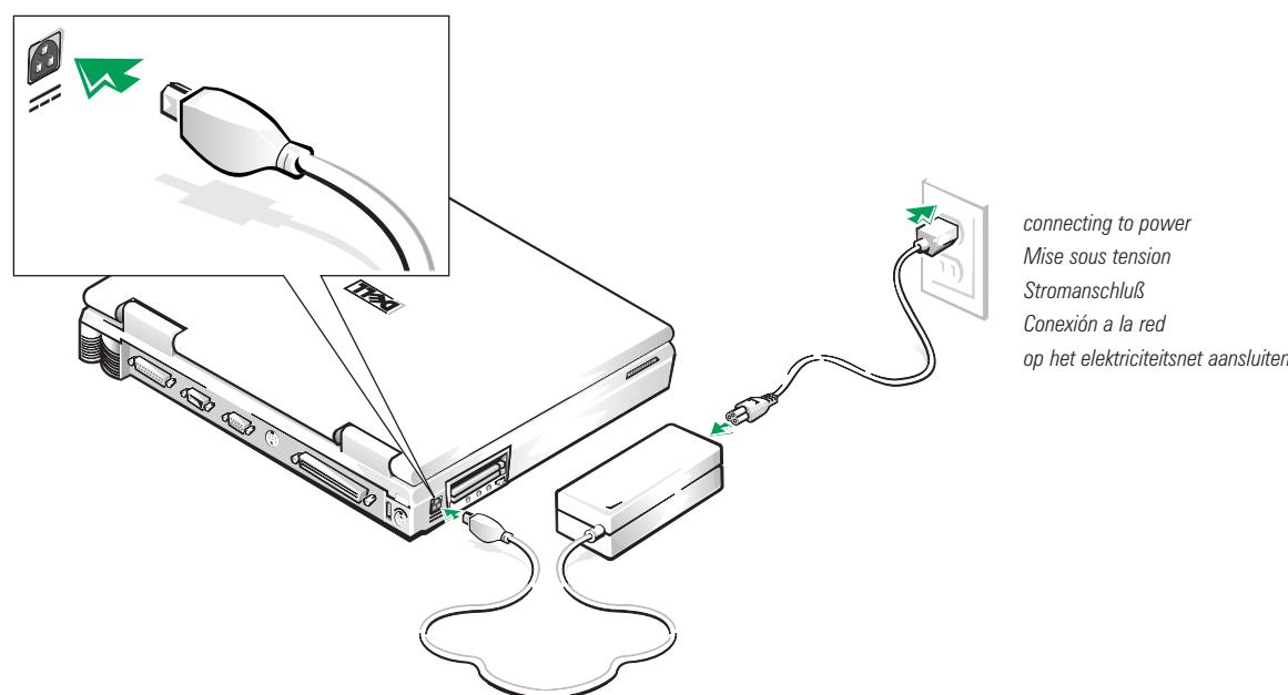
Connect the AC adapter power cable to the AC adapter. Plug the AC adapter power cable into an electrical outlet. Plug the AC adapter cable into the AC adapter connector on the computer. The green light on top of the AC adapter should light up.
