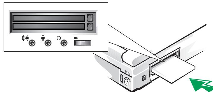
To install a PC Card, hold the card with its orientation symbol pointing into the slot and the top side of the card facing up. Insert the card into the slot and press in firmly.
