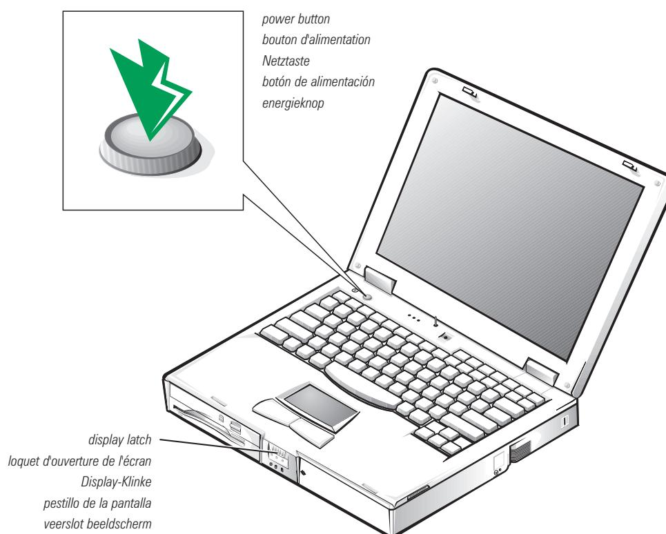
Before you turn on the computer, find the product key on the front of the Microsoft operating system book you set aside in step 2. Then open the computer display, and press the power button to turn on the computer. Use the instructions in the *Dell Inspiron Systems Setup Guide* to complete the setup of the computer.
