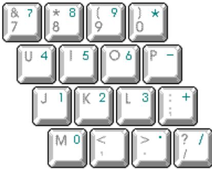
To activate the embedded numeric keypad, press <Num Lock>. The Number Lock indicator lights up.
