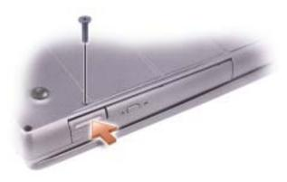
4 Pull the device out of the module bay.
