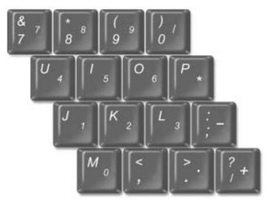
**NOTE:** When you connect an external keyboard or keypad to the computer, the keypad is disabled.
