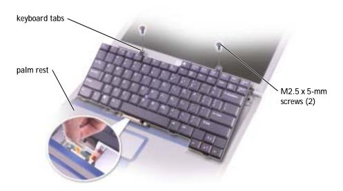
**NOTE:** When you replace the keyboard, ensure that the keyboard tabs are completely in place to avoid scratching the palm rest.
