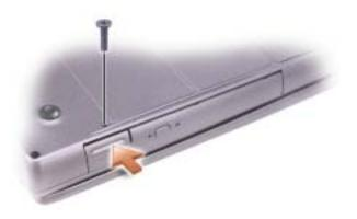
3 Pull the device out of the module bay.
