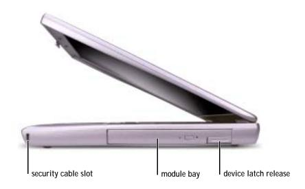
SECURITY CABLE SLOT — Lets you attach a commercially available antitheft device to the computer. For more information, see the instructions included with the device.
