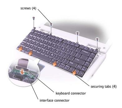
**9** Insert the four securing tabs on the keyboard into their respective slots in the palm rest, and lower the keyboard into the bottom case.
