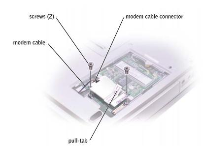
**2** Connect the modem cable to the modem.
