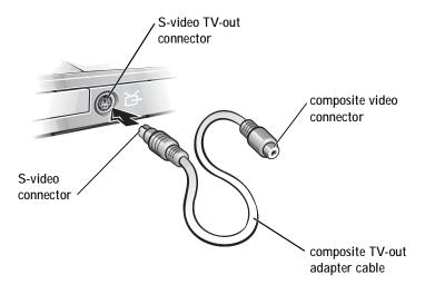
3 Plug one end of the composite video cable into the composite video connector on the composite TV-out adapter cable.
