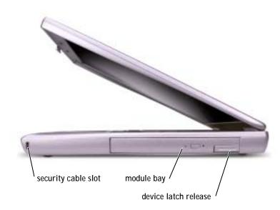
SECURITY CABLE SLOT — Lets you attach a commercially available antitheft device to the computer. For more information, see the instructions included with the device.
