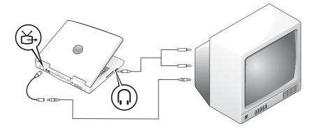
To connect the computer to a television that has a composite video input only, Dell provides a composite TV-out adapter cable. Before you begin, ensure that you have the following cables:
