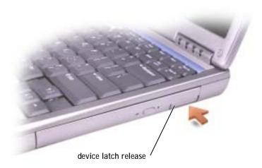
2 Pull the device by the latch release to remove the device from the module bay.
