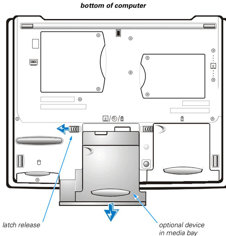
**Figure 1-1. Removing a Device From the Media Bay**
