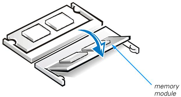
**Figure 1-6. Installing a Memory Module**
