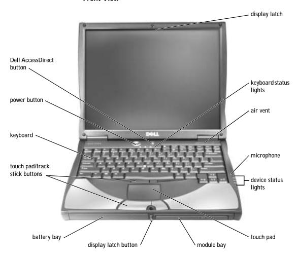
**DISPLAY LATCH** — Keeps the display closed.
