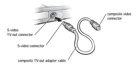
Plug one end of the composite video cable into the composite video connector on the composite TV-out adapter cable.
