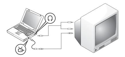
To connect the computer to a television that has a composite video input only, Dell provides a composite TV-out adapter cable. Before you begin, ensure that you have the following cables:
