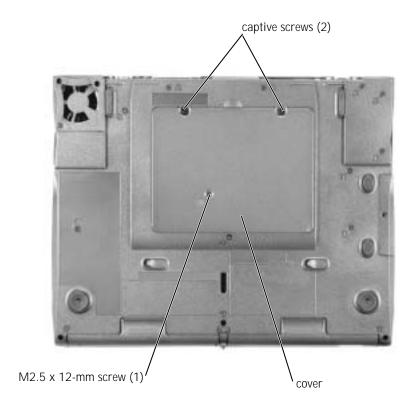
7 Remove the screw(s) from the cover, and lift up the cover.
