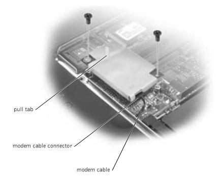
**11** Connect the modem cable to the modem.
