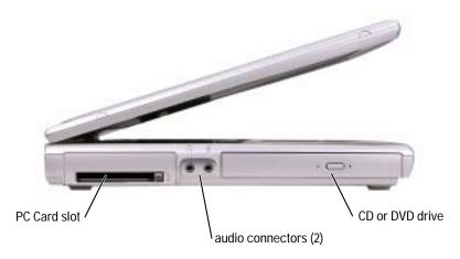
PC CARD SLOT — Supports one PC Card, such as a modem or network adapter. For more information, see "Using PC Cards" in the *Dell Inspiron Help* file. To access the help file, see page 16.
