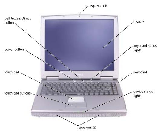
**DISPLAY LATCH** — Keeps the display closed.
