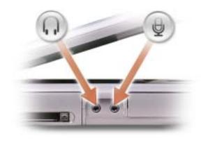
Attach headphones or speakers to the  $\bigcap$  connector. Attach a microphone to the  $\ \ \ \ \ \ \ \ \ \ \ \ \ \ \ \$  connector.
