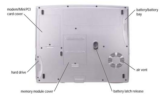
MODEM/MINI PCI CARD COVER — Covers the compartment that contains the modem and Mini PCI card. See page 82.
