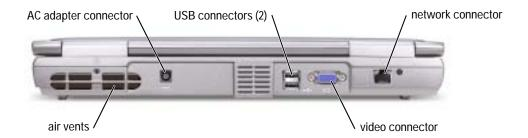
AIR VENTS — The computer uses an internal fan to create airflow through the vents, which prevents the computer from overheating.
