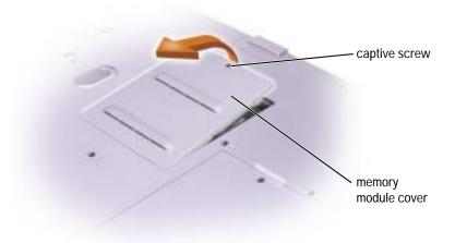
Remove the screw labeled "O" next to the memory module cover.
