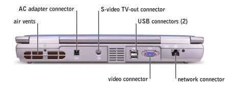
**AIR VENTS** — The computer uses an internal fan to create airflow through the vents, which prevents the computer from overheating.
