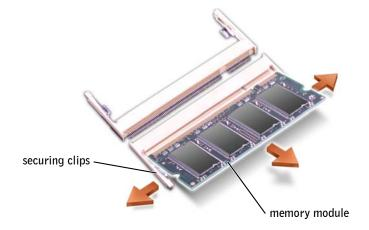
**NOTE:** If the memory module is not installed properly, the computer may not boot properly. No error message indicates this failure.
