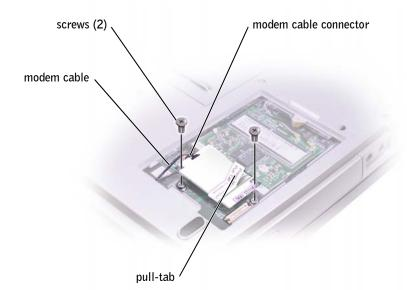
**4** Connect the modem cable to the modem.
