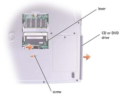
**4** Press the lever next to the memory module connectors in the direction of the arrow on the lever (towards the drive) to release the drive.
