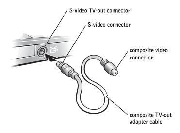
**3** Plug one end of the composite video cable into the composite video connector on the composite TV-out adapter cable.
