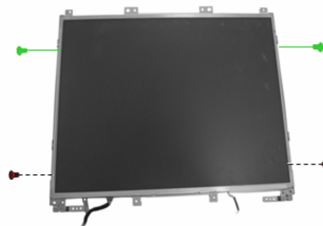
Figure 2-27 Remove 4 screws to release LCD Hinge bracket
