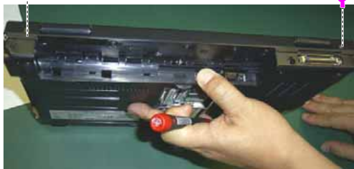
Figure 2-13 Remove 7 screws
