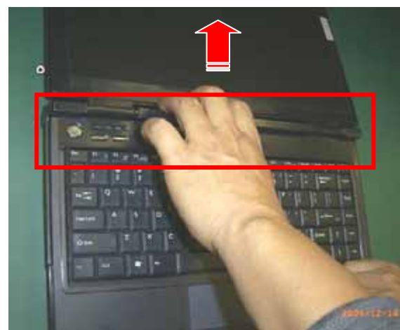
Figure2-14 Lift up the K/B Cover
