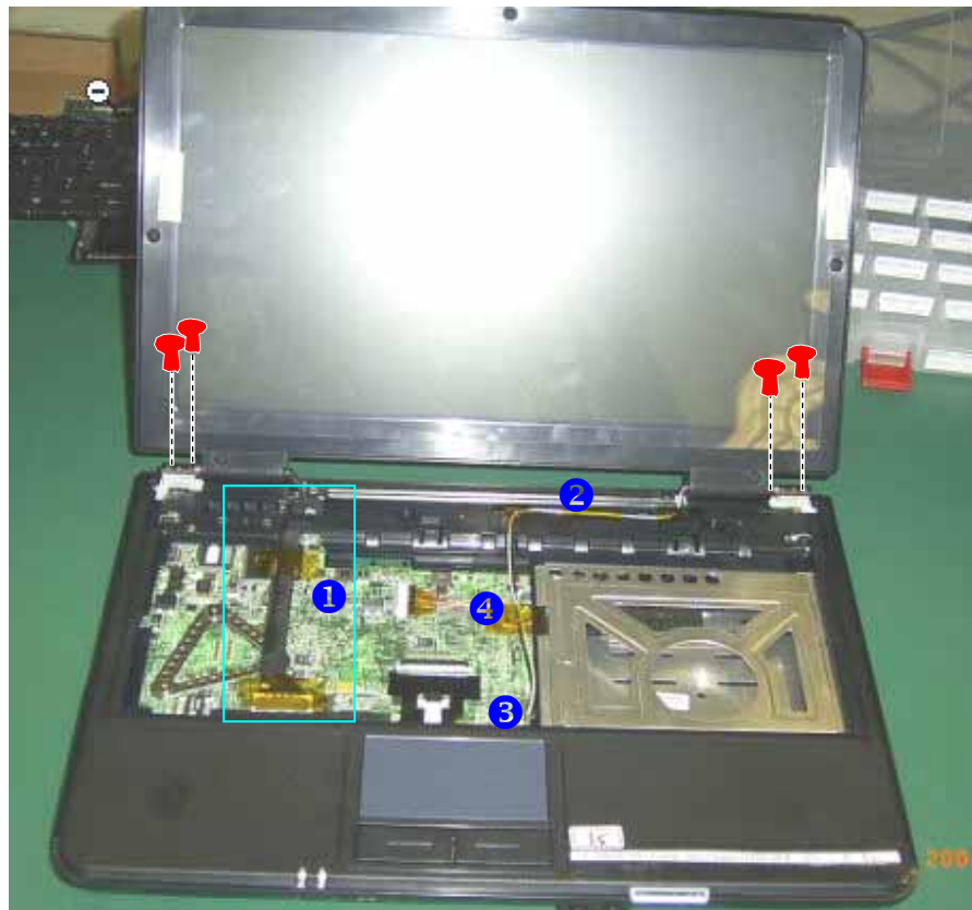
Figure 2-17 Disconnect 4 cables and remove two hinge covers with screwdriver
