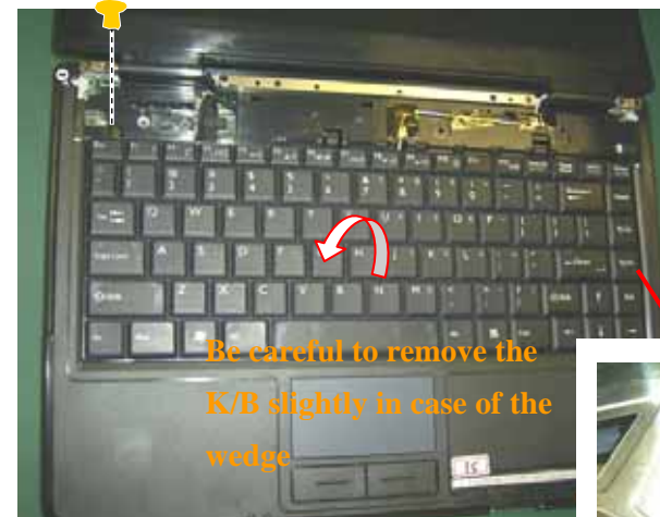
Figure 2-15 remove 3 screws and lift up the K/B
