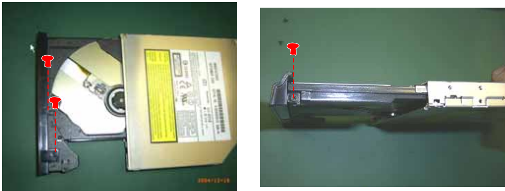
Figure 2-7 Remove 3 screws
