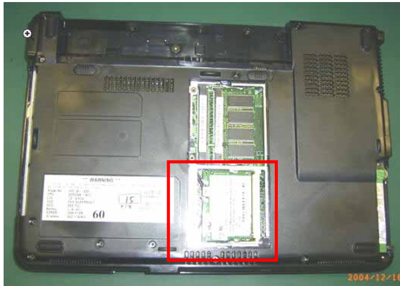
Figure 2-11 Remove the RAM Door first
