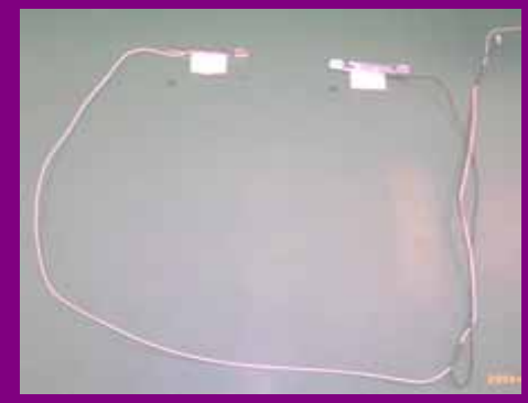
Figure 2-37 Wire antenna with bracket
