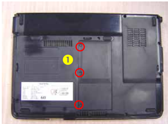
Figure 2-5 Remove the ODD Module
