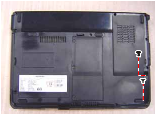
Figure 2-2 Remove the HDD cover
