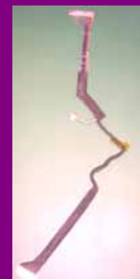
Figure 2-34 LCD FFC
