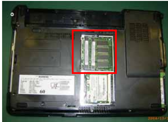
Figure 2-9 Remove the cover first
