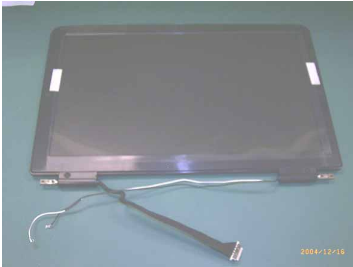
Figure 2-29 S52 LCD Module
