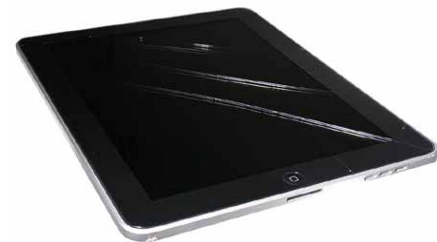
Corner dent resulting in multiple cracks.
