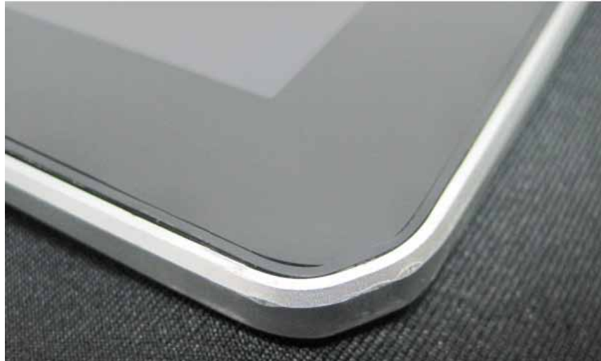
Corner dent resulting in multiple cracks.
