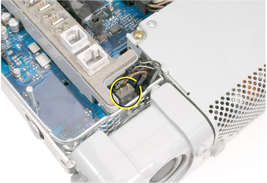
Does your computer start up when holding the screwdriver to these two contact points?
