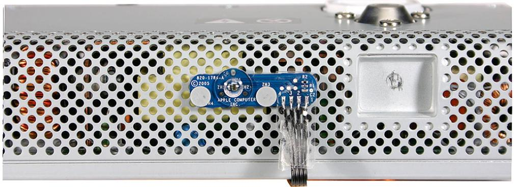
3. Locate the notched-out area (circled) on the logic board. As you lower the power supply into the chassis, make sure the ambient light sensor cable lines up with notch.
