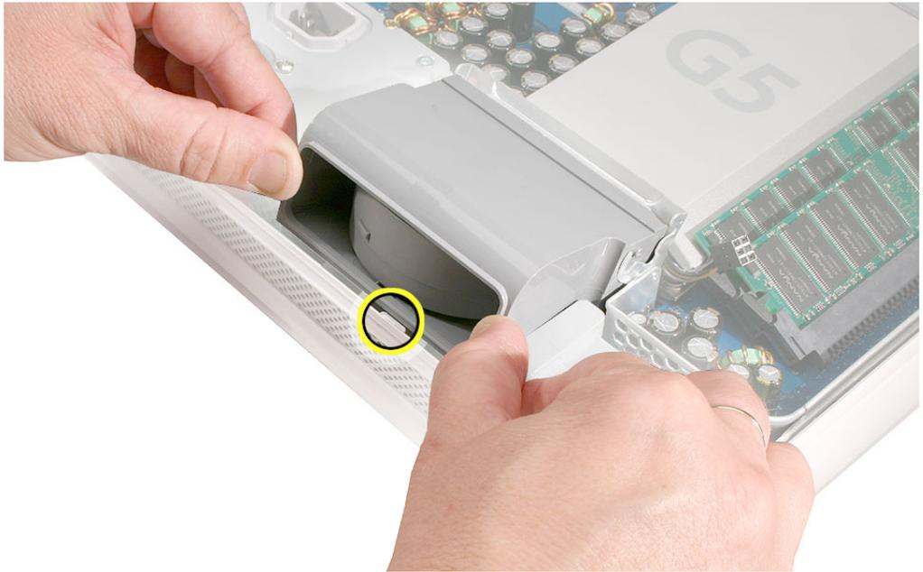
6. Pull the fan cable through the metal bracket (1) as you pull the fan forward (2).
