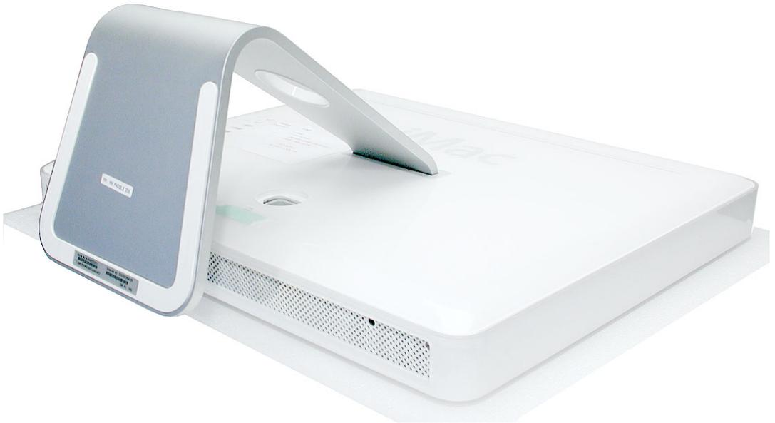
4. Locate the three silver case screws circled below. You may have to lift the stand to locate the middle case screw. **Note:** These screws are captive; they are part of the display/bezel assembly and cannot be removed.
