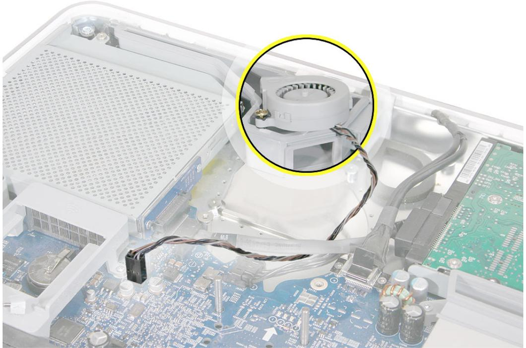
2. Place the two screws into the grommets on the replacement fan. Position the fan into place and tighten the two fan screws
