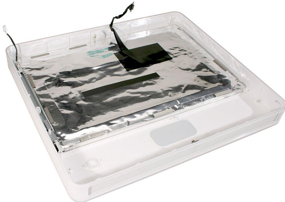
2. Make sure that the TMDS cable is tucked into the groove on the bezel as shown. A cutout on the midplane chassis lines up with the groove on the display/bezel assembly housing
