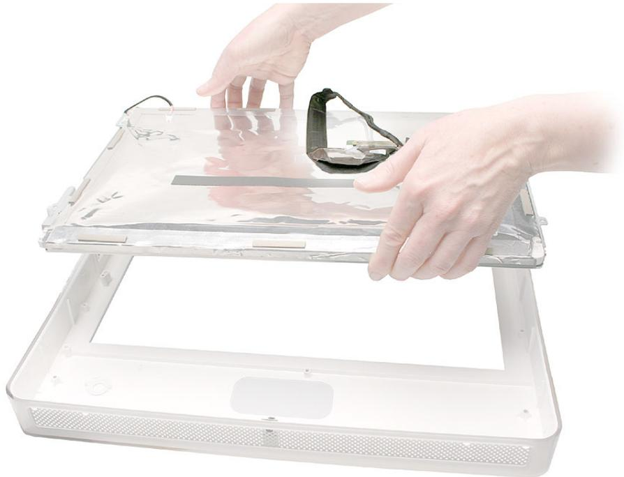
3. Place the LCD panel into the display bezel so that all four screw holes on the brackets align with the screw holes on the bezel.
