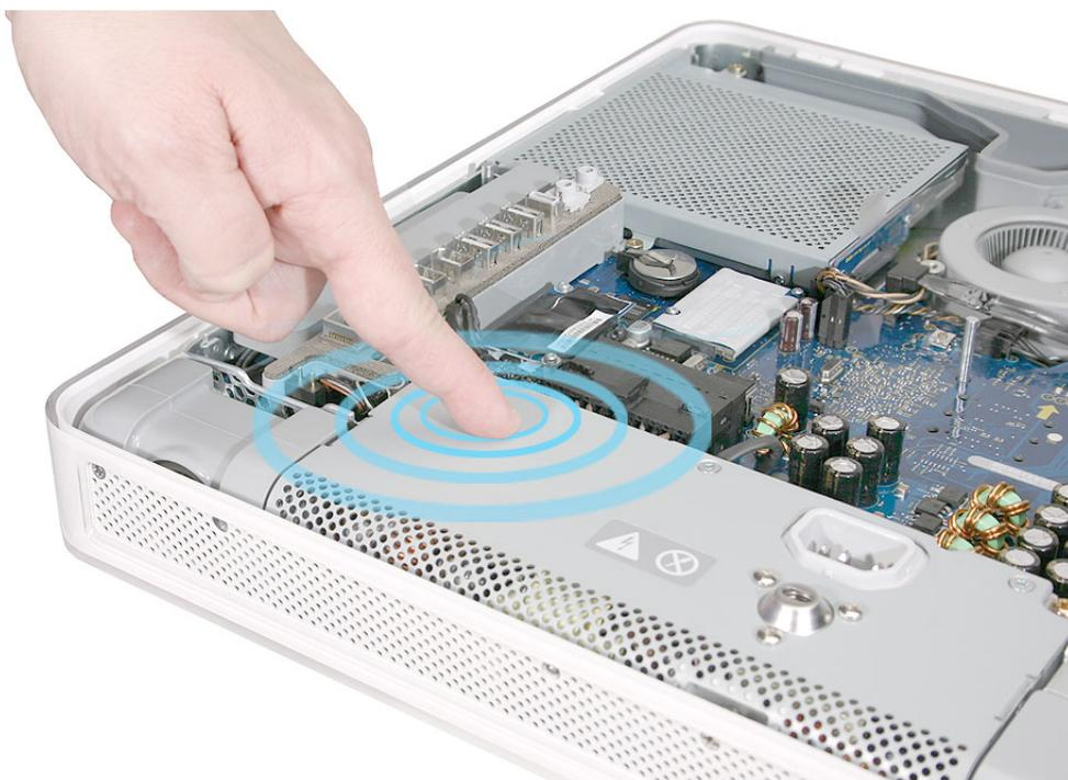
3. Locate the fan cover near the top of the computer.
