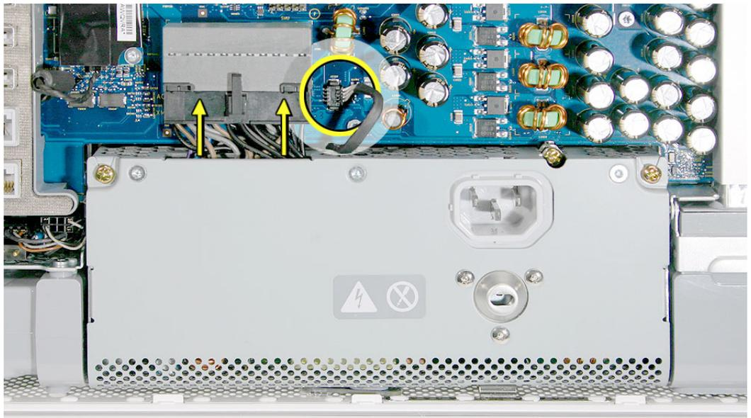
8. Tighten the two outer captive screws.
