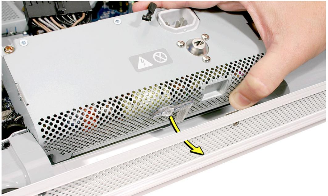
6. Once the power supply is installed, check that the ambient light sensor cable is positioned in the notched-out area on the board.
