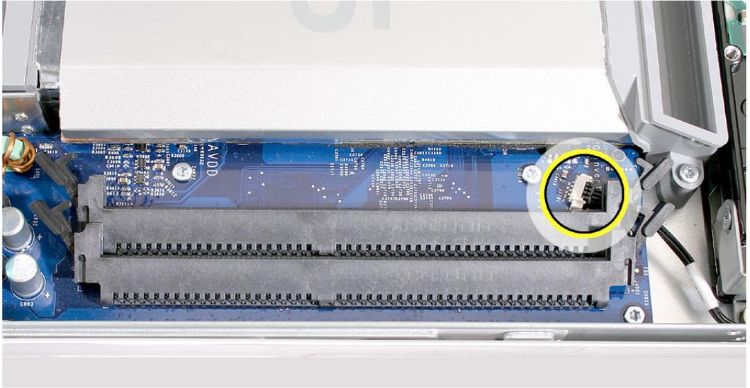
14. Using a T-8 screwdriver, connect the two fan duct screws. **Note:** These two screws are longer than the other silver screws securing the logic board to the midplane chassis.
