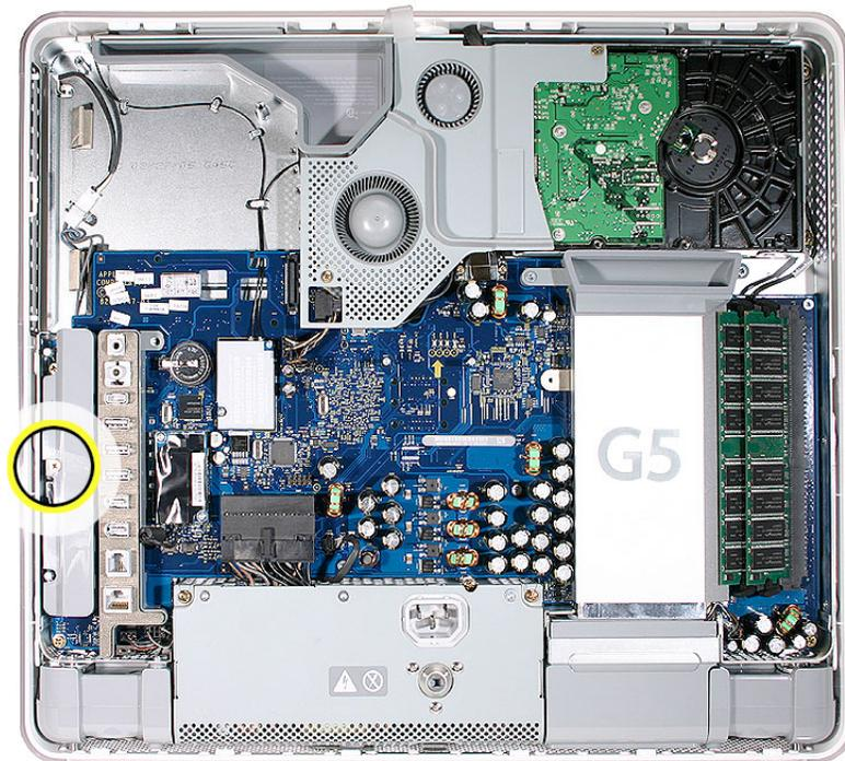
5. Lift the inverter straight up to disconnect the inverter board.
