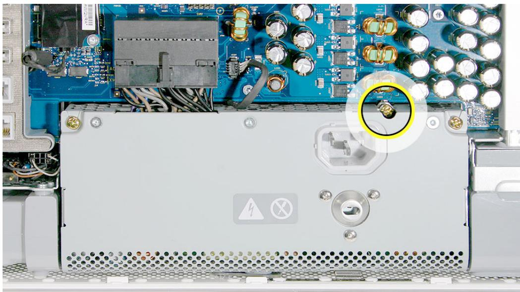
10. Turn the middle case screw to the left about five revolutions. This step prepares the back cover for installation.
