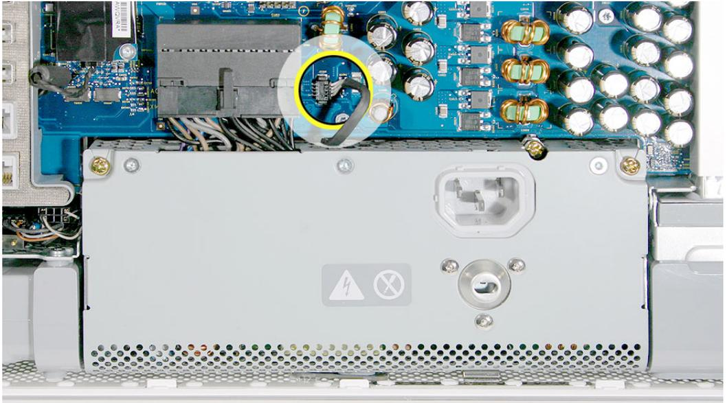
4. Turn the middle case screw clockwise about five revolutions. This releases the back cover clamp screw.
