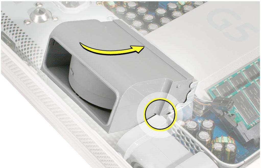
3. As you push the fan, make sure it clears the white tab on the display bezel.
