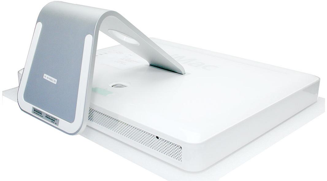
4. Raise the foot and use a Phillips #2 screwdriver to loosen the three screws at the bottom of the computer by turning them to the left. These are “captive screws,” which means they’re not supposed to come all the way out.
