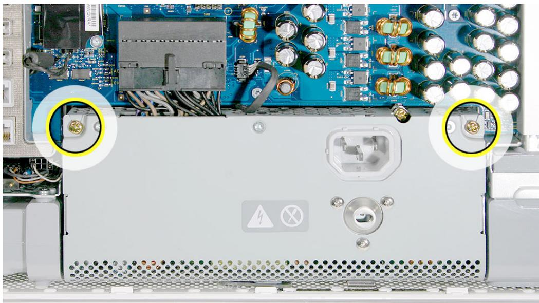
9. Tighten the last captive screw (circled) that attaches to the display bezel.
