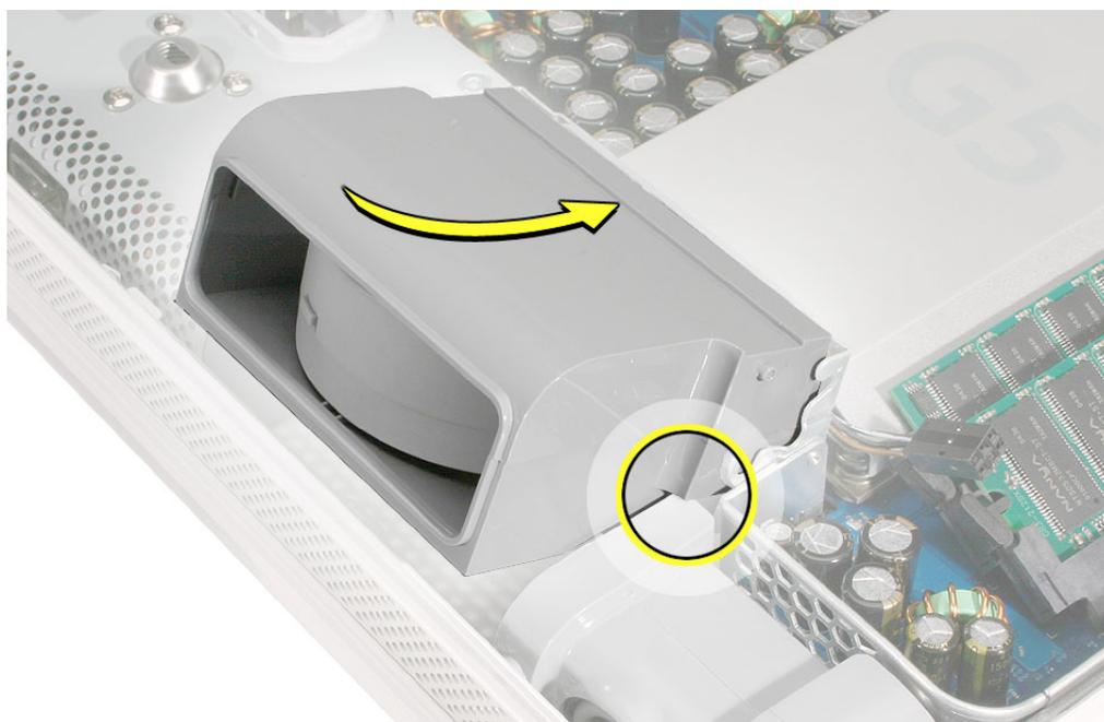
3. As you push the fan, make sure it clears the white tab on the display bezel.
