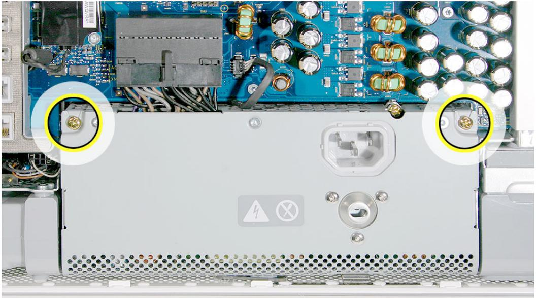
2. Loosen the middle captive screw (circled) until it's flush with the top of the power supply. This screw attaches to the display bezel; make sure to loosen it all the way.
