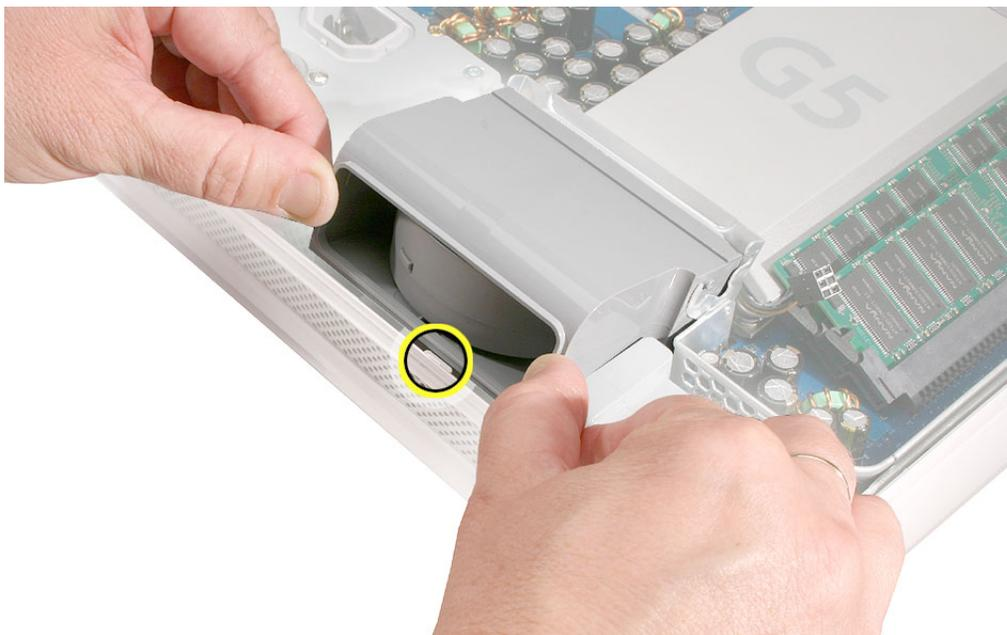
6. Pull the fan cable through the metal bracket(1) as you pull the fan forward (2).
