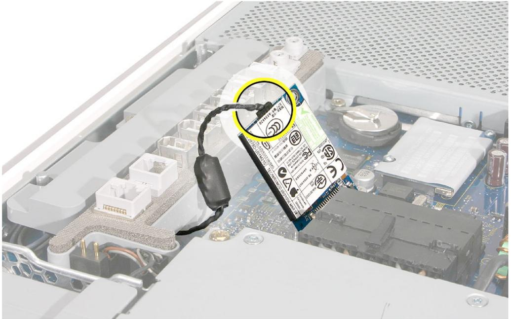
2. Press the board onto the connector. Replace the two T-6 screws on the board.
