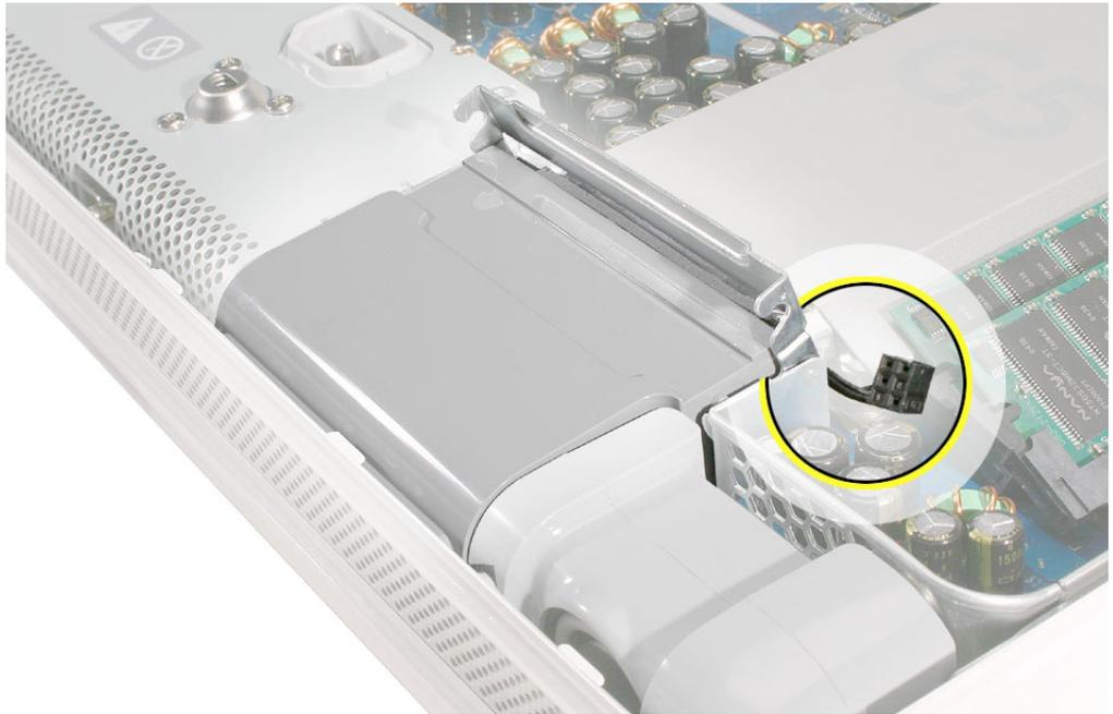
4. Grab the fan by the sides and wiggle the fan upward. As the fan comes up, it will bump into a tab on the front bezel. See the next step.
