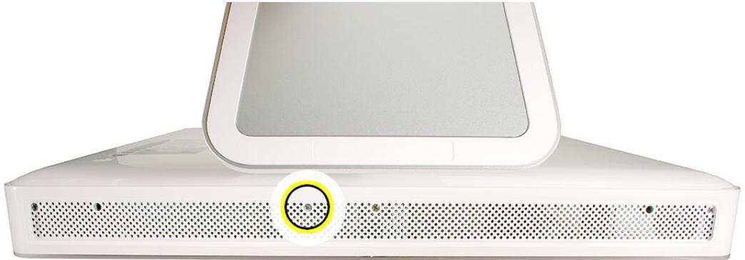
The ambient light sensor attaches to the power supply with two plastic rivets.
