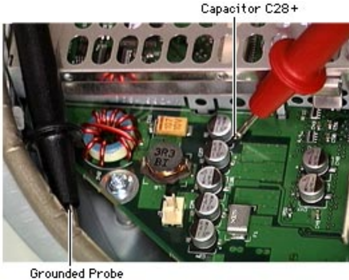
Testing for Power at the Logic Board
