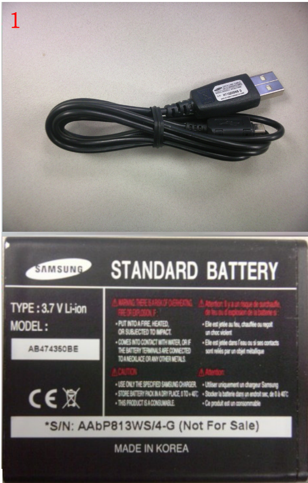
USB Data Link Cable : BENU to PC (GH39-00922A) Standard Battery for BENU (GH43-02986A)
