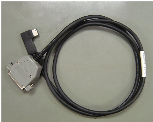
3. Test cable (1.5M:GH39-01011A / 0.4M:GH39-01013A) :JIG to phone
