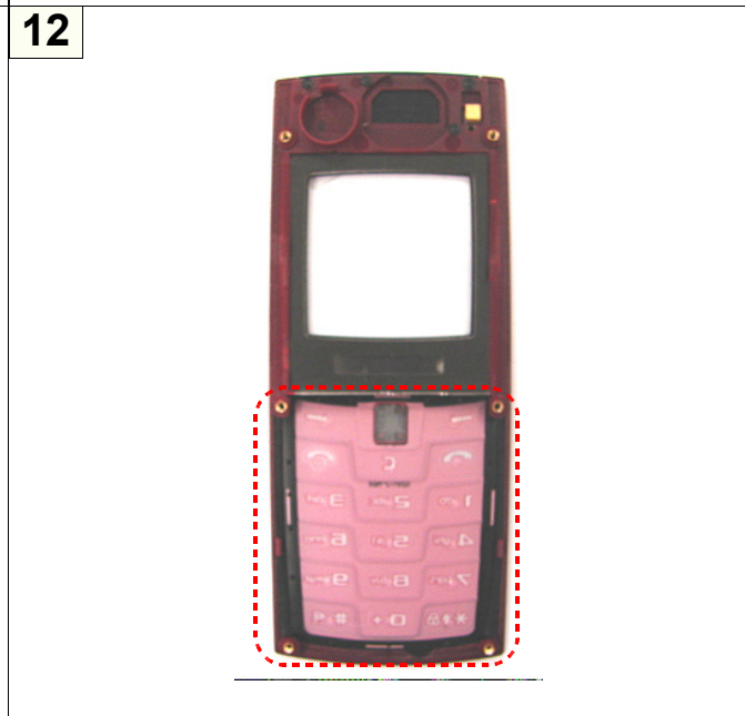
Assembly of KEY PAD Put KEY PAD into the FRONT as you see above.
