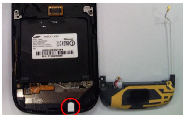
1.Unscrew and Disassemble Speaker and MIC HOLDER.
