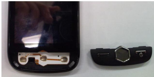
1.Disassemble KEY PAD like the picture.
