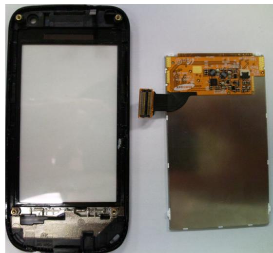
1. Disassemble LCD Bracket.(Read Mark: HOOK Point)
