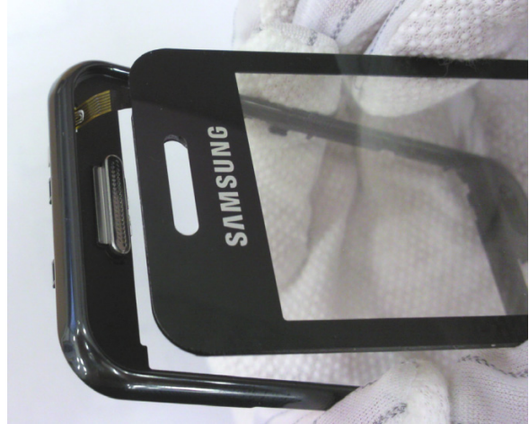
Insert TSP FPCB through the FRONT's hole carefully when assembling FRONT and TSP. (Refer to the picture.)
