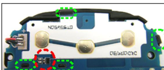
**4** 1) Assemble the SHIELD CAN.
