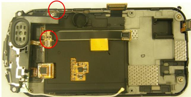
1) Make sure not to damage the connector and the FPCB.
