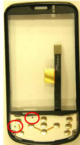
1) Make sure the absorber is fit inside the border.
