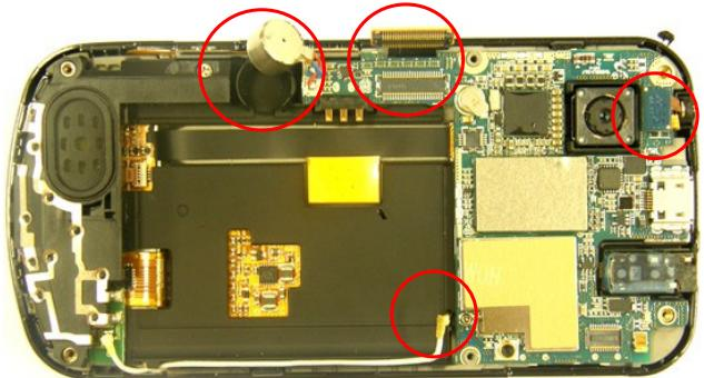
1) Disconnect the connector of SUB PBA from the Main PBA and remove the tape
