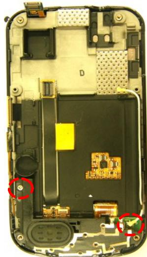
1) Make sure not to damage the FPCB while inserting it.
