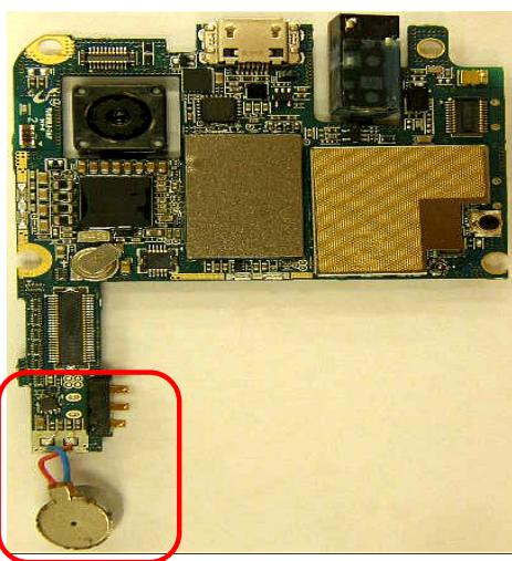
1) Make sure not to damage Camera FPCB
