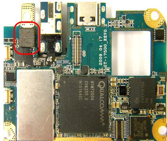
1) Make sure not to make any damage on the shield cans.
